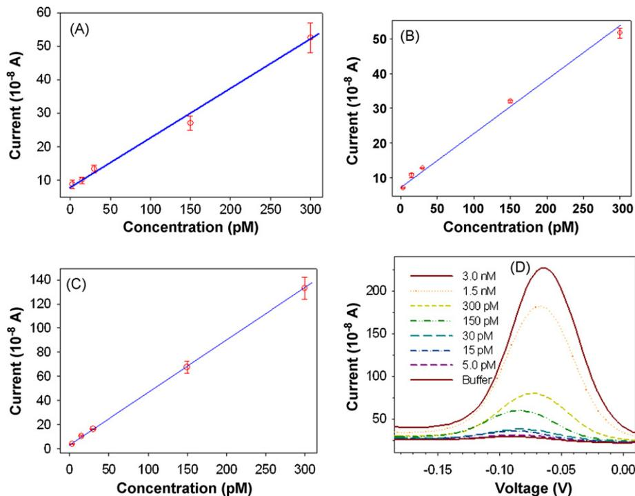
**Fig. 1.** Results of the three sandwich strategies based electrochemical immunoassay of nitrated fibrinogen. (A), (B) and (C) are the calibration curves of current peak height as a function of the concentration of nitrated fibrinogen from strategy A, strategy B and strategy C, respectively. (D) Voltammograms of nitrated fibrinogen with increasing concentration from bottom to top (strategy B).
