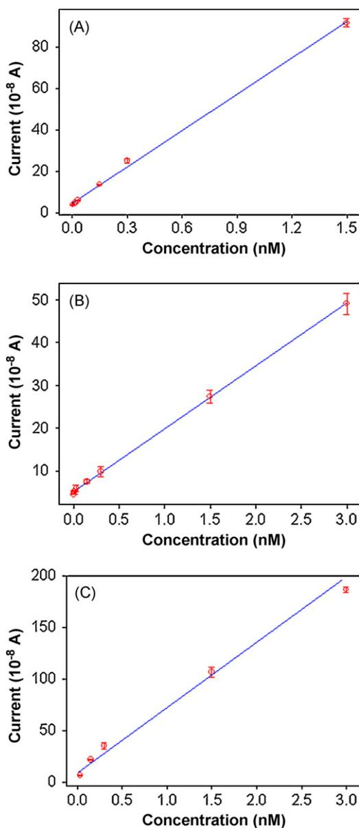
**Fig. 5.** Strategies B and C based electrochemical immunoassay of nitrated fibrinogen spiked in human plasma and serum. (A) and (B) are calibration curves of strategy C assay of human serum samples and plasma samples, respectively. (C) Calibration curve of strategy B assay of human plasma.
