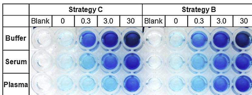
**Fig. 4.** The image of developed plate using optimized conditions. The blank samples means there were no immunoreactions in these wells. The concentration of spiked nitrated fibrinogen was labeled in nM. The samples were prepared in 0.5% BSA (top), 20 times diluted human serum in 0.5% BSA (middle) and 20 times diluted human plasma in 0.5% BSA (bottom).
